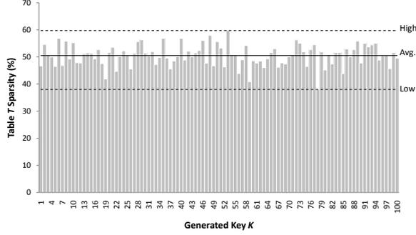
Fig. 3. Fraction of table  $T$  logic value 0s for 100 generated keys  $K$
