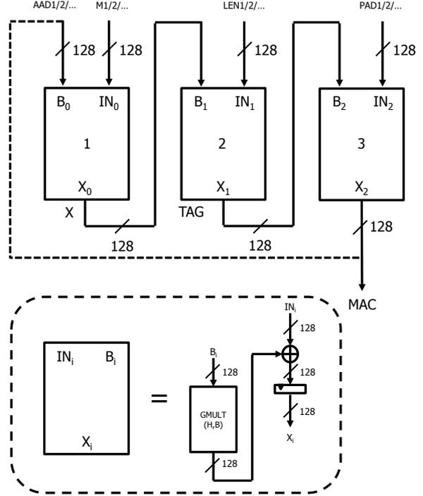
Fig. 4. A multi-stage pipelined GHASH module implementation. The bottom of the figure shows the structure of one pipeline stage
