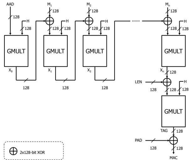
Fig. 1. Block diagram of a combinational implementation of the GHASH function.
